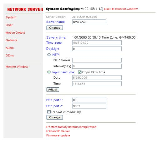
To set an additional port for accessing the Lorex Monitor, click on the 'System' link. The following screen will appear;
